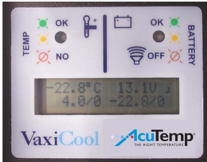
Figure 6. The LCD and LED Panel
